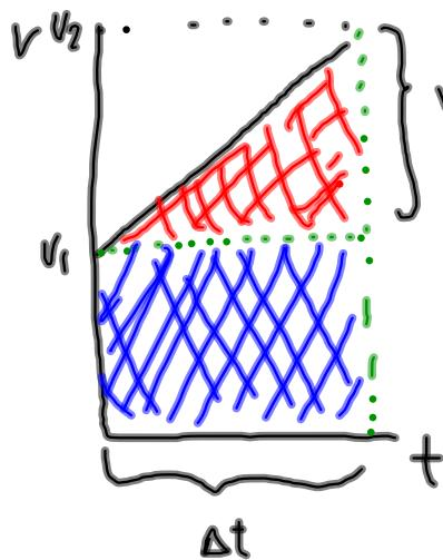
$$\begin{aligned} \text{Area of trapezoid} &= \boxed{\text{square}} + \triangle \\ &= b \times h + \frac{1}{2} b \times h \\ &= v_1 \Delta t + \frac{1}{2} (\Delta v) (\Delta t) \end{aligned}$$
